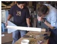
Drilling the bulkhead mount.
