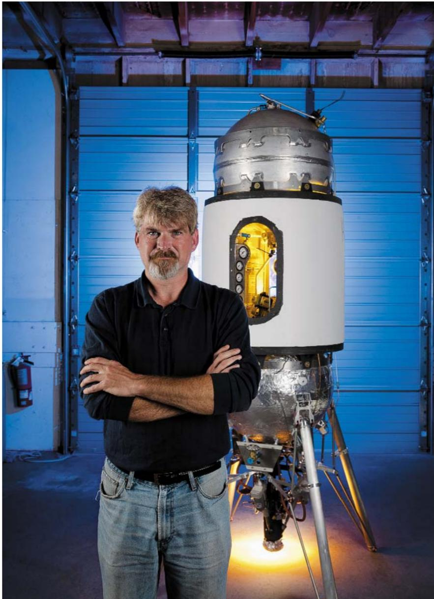
Xombie is even hotter in person: A reusable vertical-takeoff/vertical-landing vehicle, about the height and girth of an industrial water heater, with four landing struts and a single liquid oxygen/isopropyl alcohol engine. Xombie is the test horse for big sister Xaero, scheduled to offer commercial lifts into a high-quality microgravity environment (like that on an orbiting space shuttle, as opposed to high-altitude balloons or sounding rockets) sometime this year.
